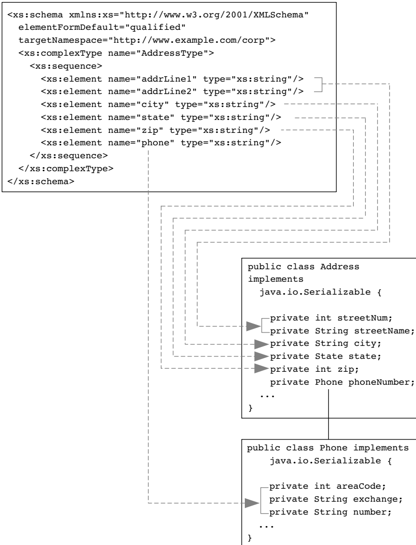
Figure 4-7 A type mapping for the Address XML Schema definition to the Address Java class definition.
